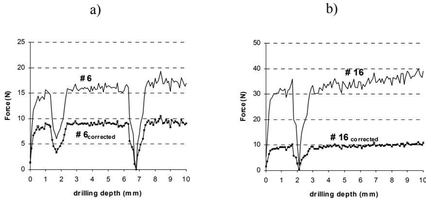
**Figure 8:** Correction of drill plots where simulated zones with very low drilling resistance were introduced in actual SV curves. Plots for holes # 6 (left) and # 16 (right) before and after correction
