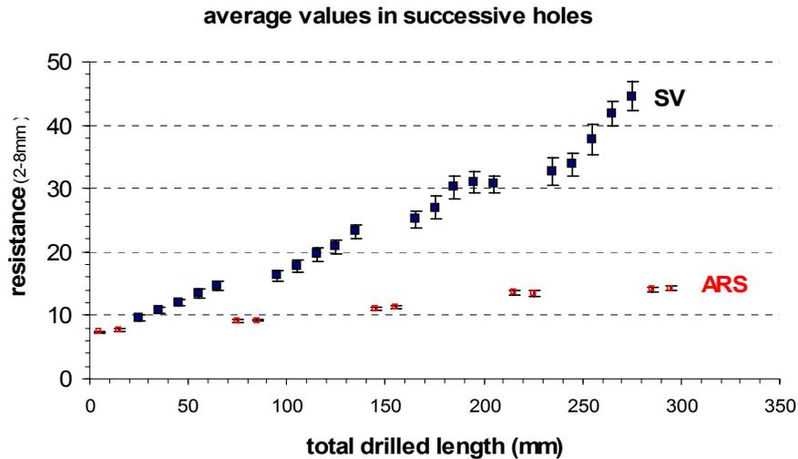
**Figure 2:** Evolution of mean resistance values on Sander specimens and on ARS due to drill bit wear. The drilled lengths on both materials are added in this representation
