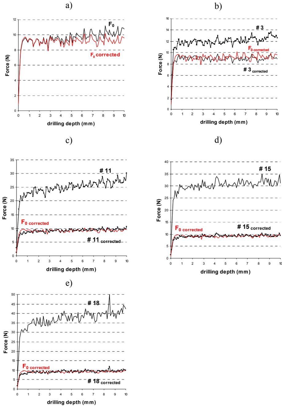
**Figure 7:** Examples of SV plots. a)  $F_0$  plot before and after correction; b), c) and d), respectively, holes # 3, #11, # 15 and #18 before and after correction, compared to the corrected  $F_0$  plot. The plots to be corrected were taken one from each of the four different wear rates.
