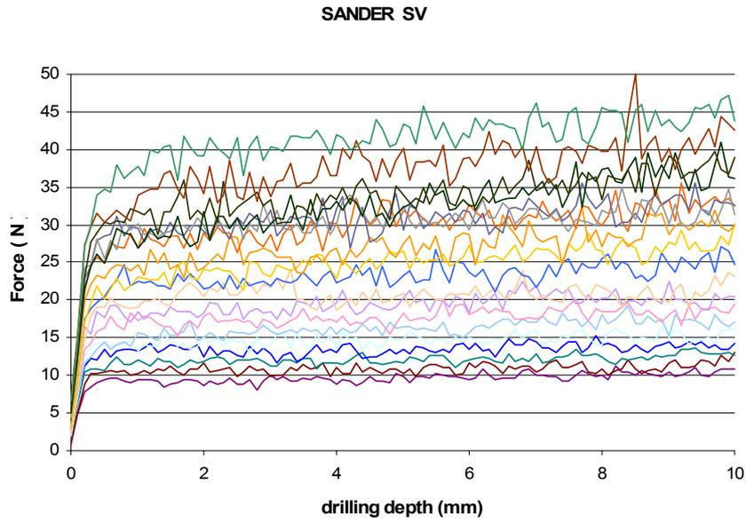
Figure 5: Original plots of 19 holes in Sander sandstone (SV) before correction
