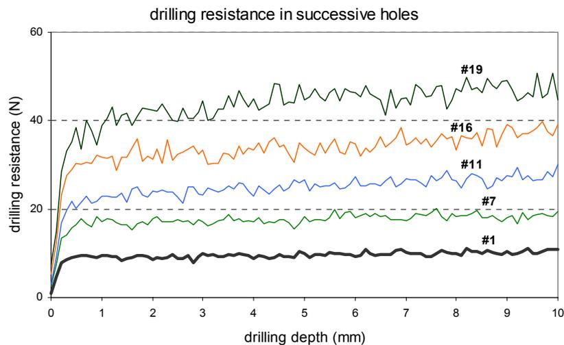
**Figure 1:** Drilling resistance graphs for Sander sandstone after 1, 7, 11, 16 and 19 holes made with a unique drill bit
