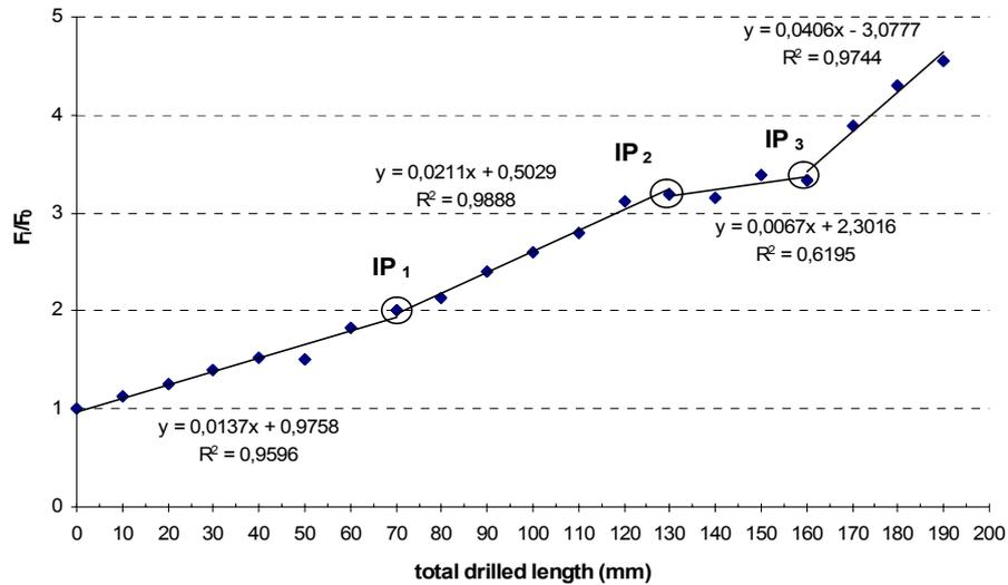
**Figure 4:** Correction functions in SV Sander sandstone. IP indicate the points where a new wear rate starts and a new set of correction parameters should be used
