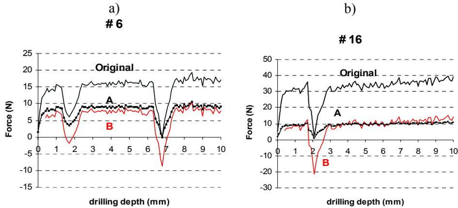
**Figure 9:** Correction of drill plots of Fig. 8 using the proposed methodology (A) compared with one subtracting formula (B). Notice the negative values obtained with the subtracting formula (B) and its absence when the new one (A) is used
