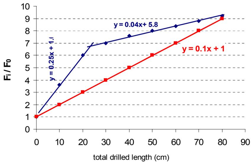
**Figure 3:** Examples of two hypothetical correction functions for two different materials
