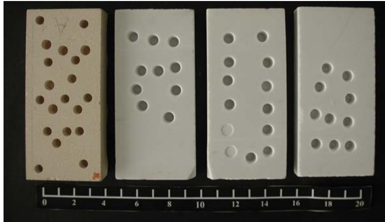
Figure 8: ARS (first on the left) and Bianco P marble samples used in the laboratory tests
