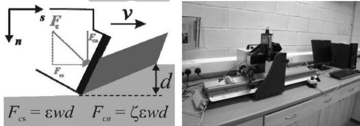
**Figure 1.** Schematic view of the cutting procedure during the implementation of a scratch test (Dagrain & Germay, 2006) (left). The Epslog Engineering WOMBAT Scratch Tool (right).
