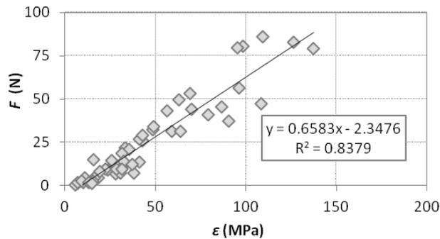
**Figure 5.** Correlation of the micro-drilling results, expressed by drilling resistance force ( $F$ ), with scratching test results, expressed by the intrinsic specific energy ( $\epsilon$ ).
