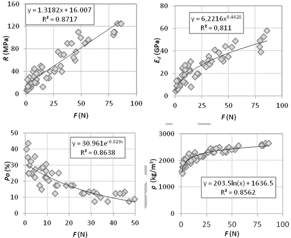
**Figure 4.** Correlation of the micro-drilling results, expressed by drilling resistance force ( $F$ ), with uniaxial compressive strength ( $R$ ), dynamic modulus of elasticity ( $E_d$ ), open porosity ( $P_o$ ) and density ( $\rho$ ).
