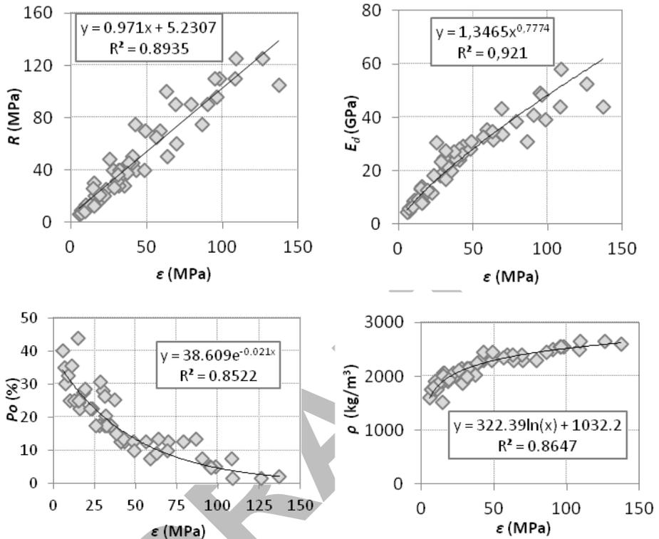
**Figure 3.** Correlation of the scratching test results, expressed by the intrinsic specific energy ( $\epsilon$ ), with uniaxial compressive strength ( $R$ ), dynamic modulus of elasticity ( $E_d$ ), open porosity ( $P_o$ ) and density ( $\rho$ ).
