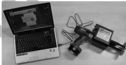
**Figure 2.** The Drilling Resistance Measurement System (DRMS).
